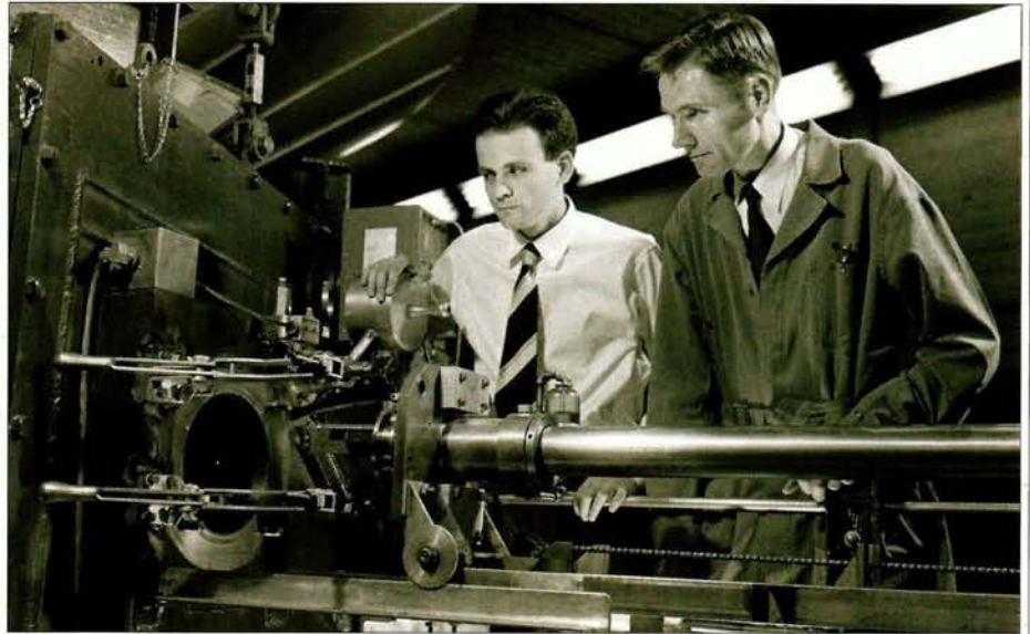
Cesare Lattes, left, with Eugene Gardner and the nuclear emulsion positioning apparatus for the 184 inch cyclotron. (Courtesy Lawrence Berkeley National Laboratory.)
