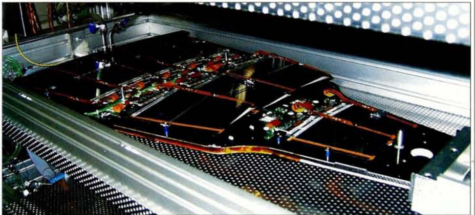
One of the CMS silicon tracker end-cap petals under test in a close-to-final environment in Lyon. (Courtesy IN2P3-CNRS Lyon.)
