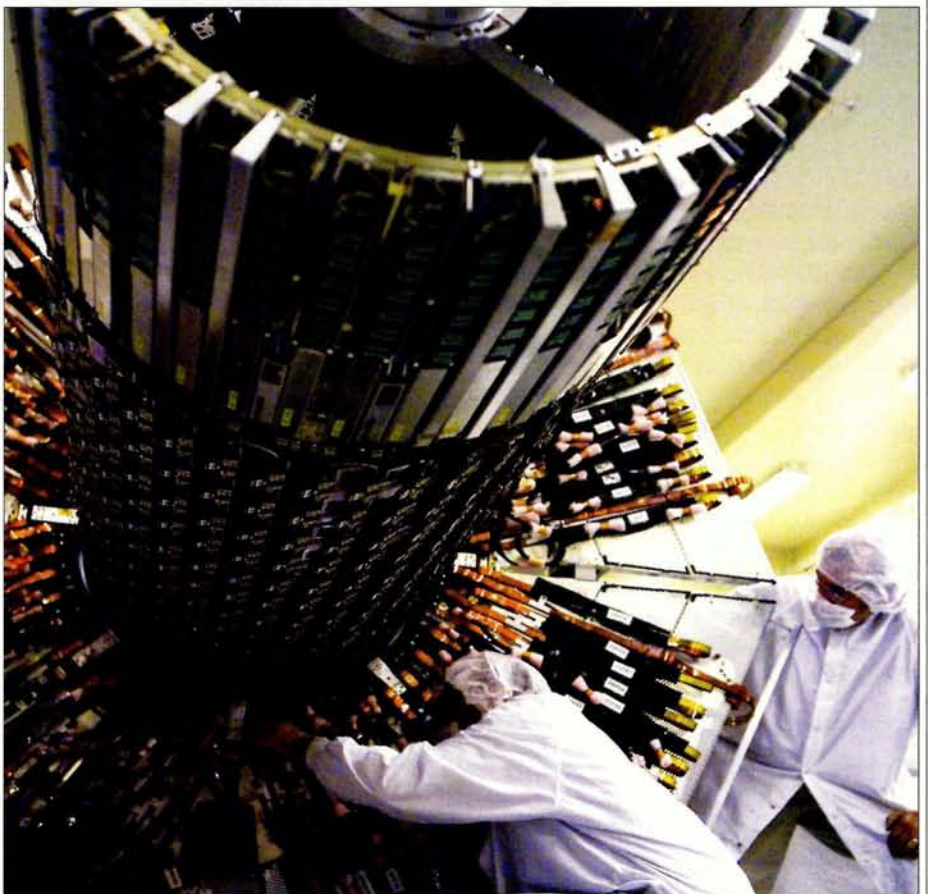
The insertion of a completed barrel of the ATLAS inner detector into its support structure.
